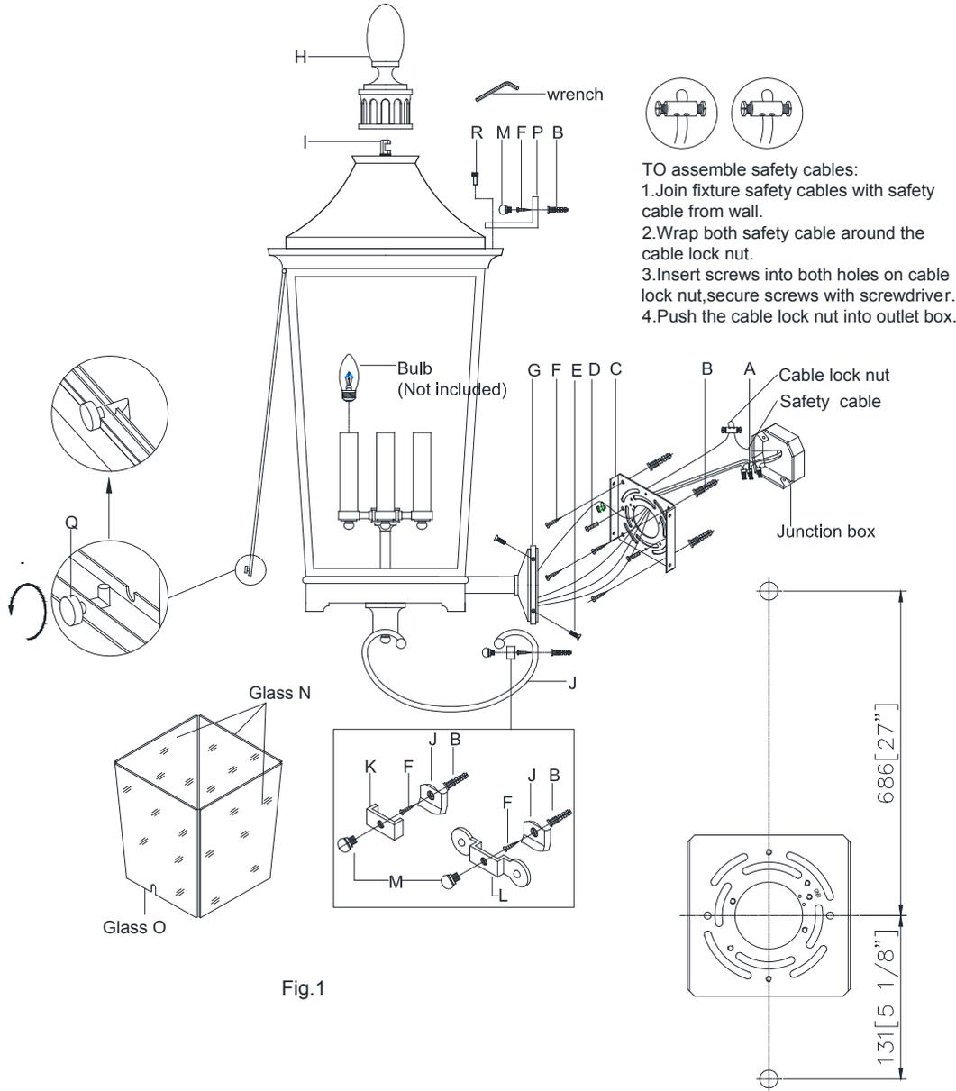
14. Attach fixture body to the bracket (P) and secure with screws (R) by using the wrench.
